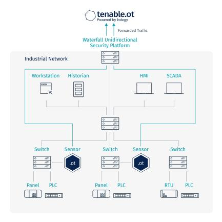
3. The Waterfall USG captures traffic from your critical network through a local mirror or SPAN port and makes that traffic available directly to an ICP (located outside of the critical network) for analysis.
